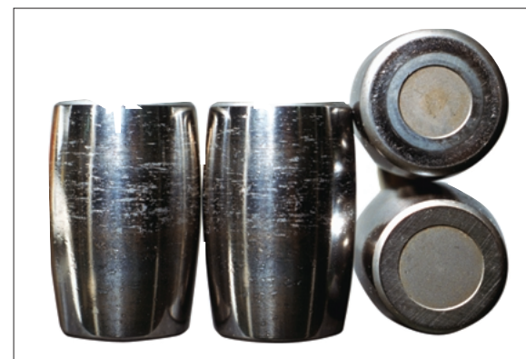
Fig. 35 Scoring on the Roller End Face
